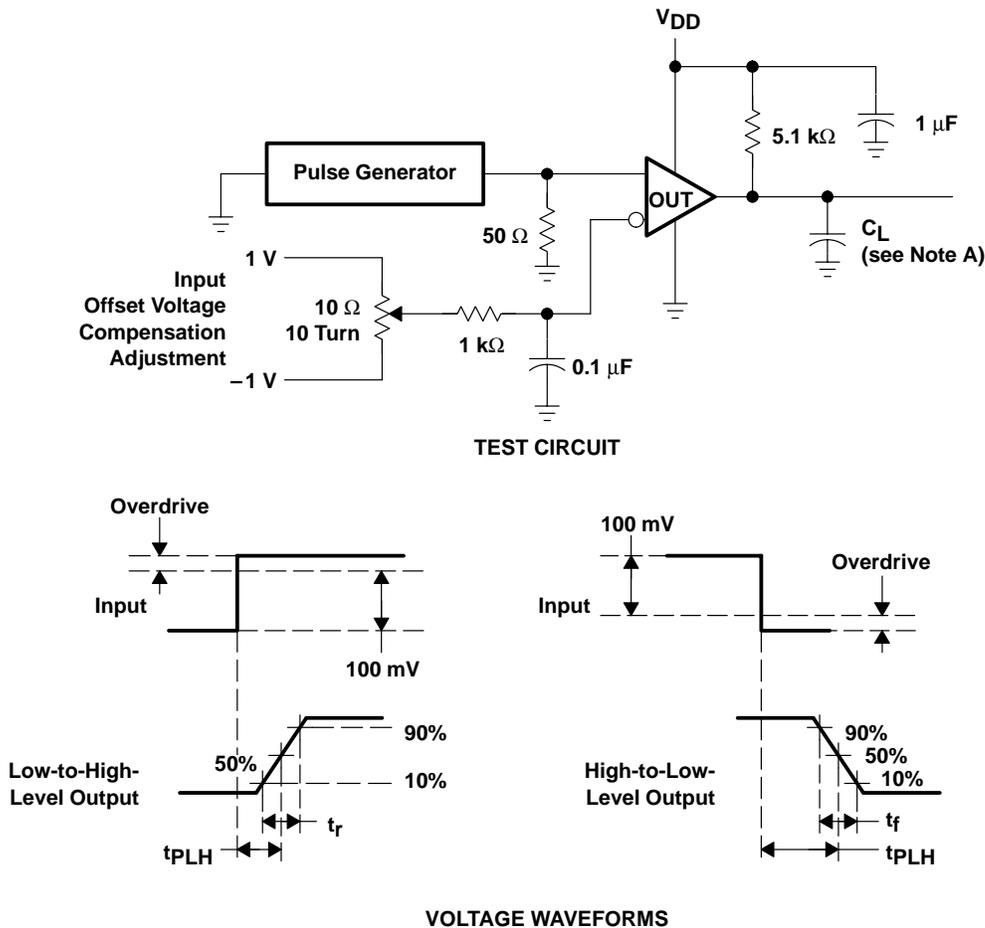
NOTE A:  $C_L$  includes probe and jig capacitance.
