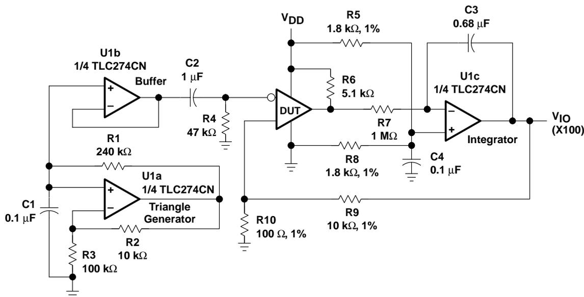
Figure 2. Test Circuit for Input Offset Voltage Measurement
