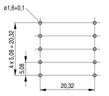
Hole arrangement View in mounting direction
