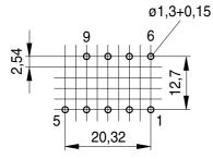
Hole arrangement View in mounting direction
