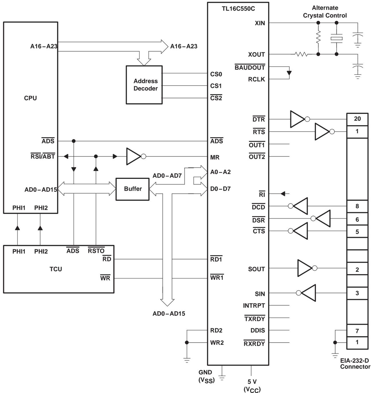
Figure 22. Typical TL16C550C Connection to a CPU
