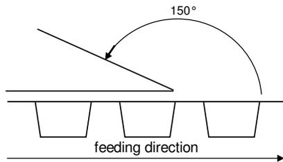
The force for tearing off cover tape is 20 to 70 grams in arrow direction
