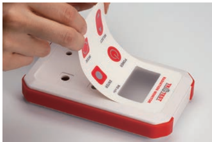
8. Sticking overlay sheet onto enclosure
