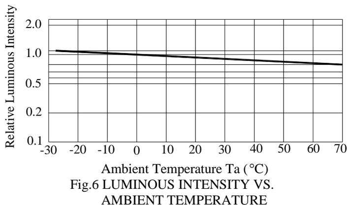
Fig.6 LUMINOUS INTENSITY VS.
