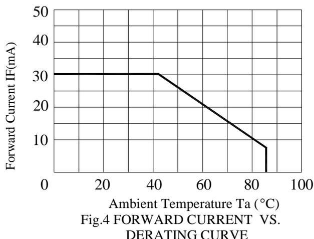
Fig.4 FORWARD CURRENT VS. DERATING CURVE
