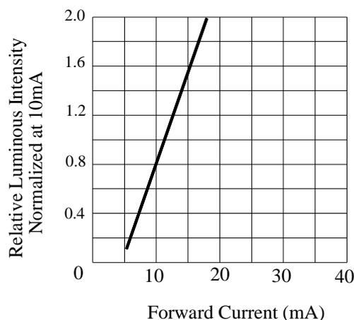
Fig.5 RELATIVE LUMINOUS INTENSITY
