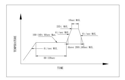
Recommended Pb free reflow soldering profile:
