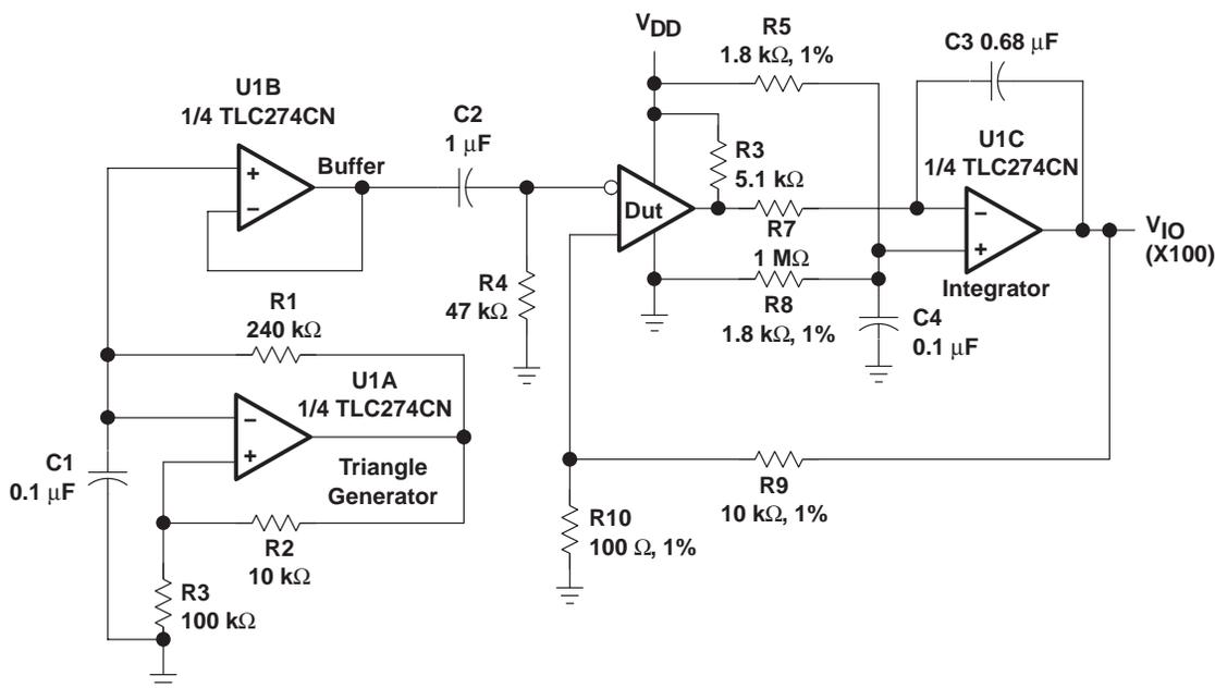
**Figure 2. Circuit for Input Offset Voltage Measurement**
