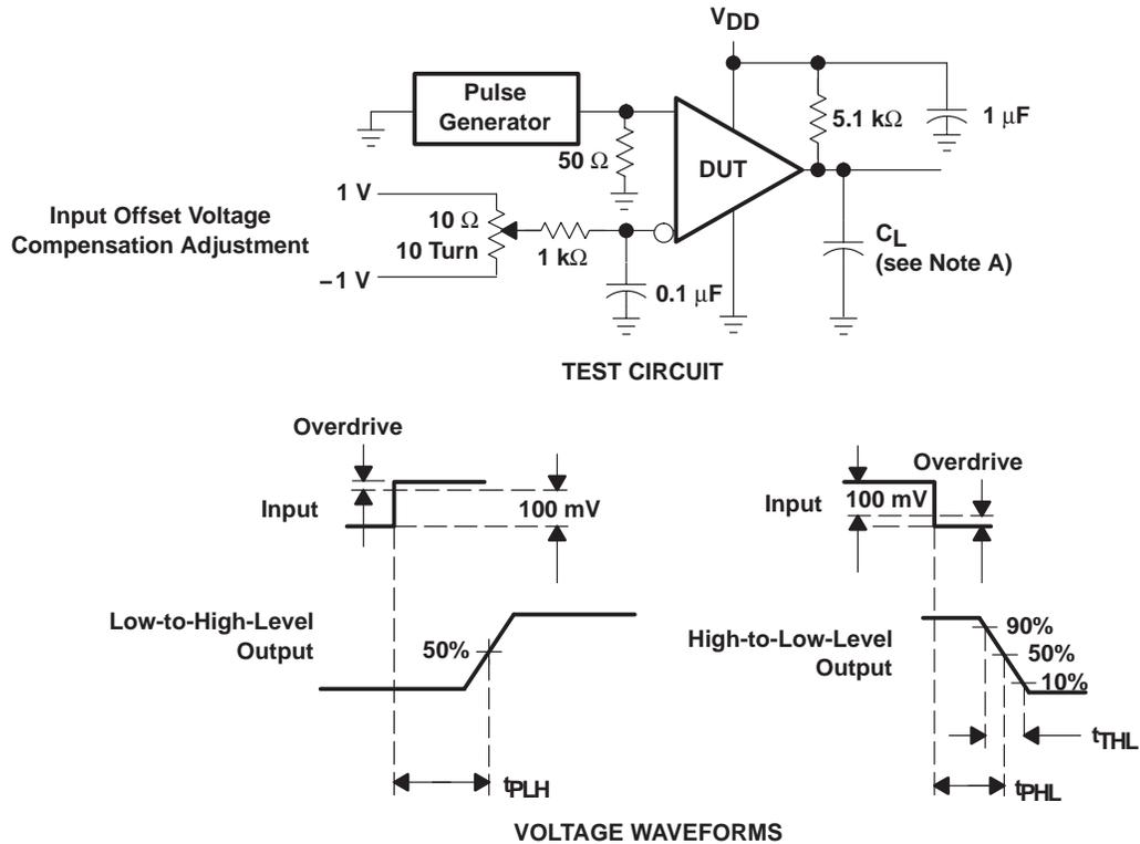
NOTE A:  $C_L$  includes probe and jig capacitance.
