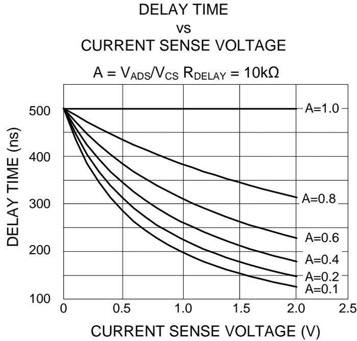
**Figure 13. Delay Time Under Varying ADS Voltages**
