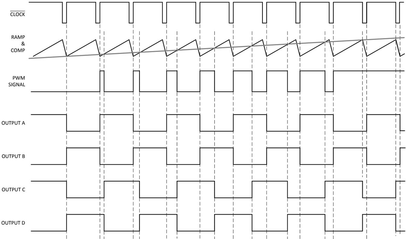
No Output Delay Shown, COMP to RAMP offset not included.
