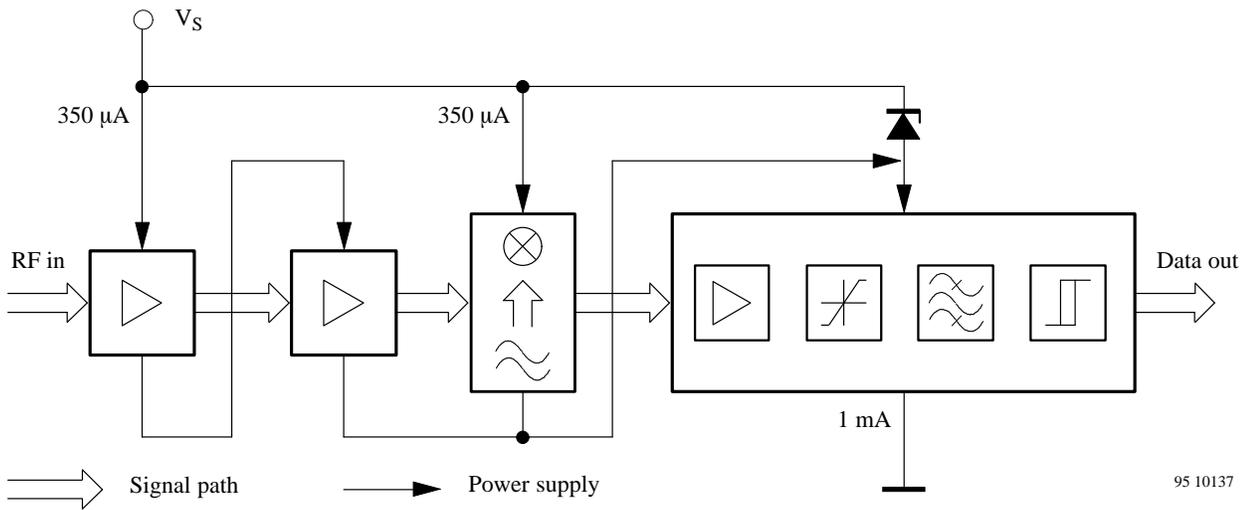
Figure 29. Principle diagram UHF remote control receiver
