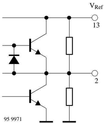
Figure 5. Pin 2 OP<sub>out</sub>
