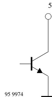
Figure 8. Pin 5 Comp<sub>out</sub>
