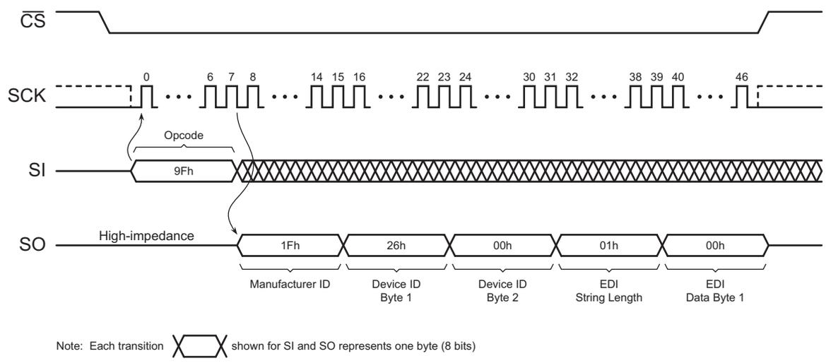
**Figure 26-11. Manufacturer and Device Read Timing (Opcode 9Fh)**
