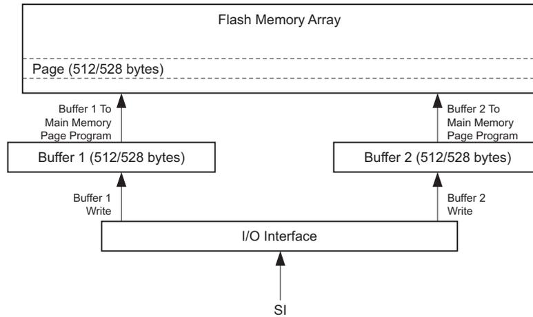
Figure 24-1. Block Diagram
