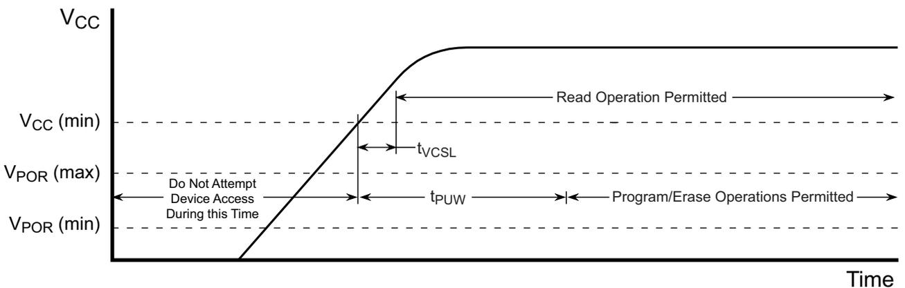
**Figure 17-1. Power-Up Timing**
