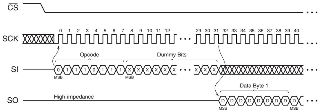
**Figure 26-9. Read Security Register Timing (Opcode 77h)**
