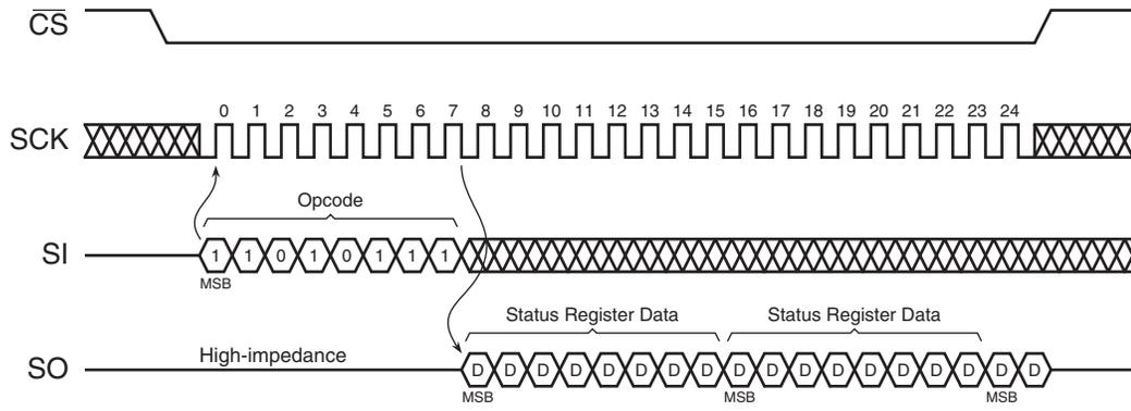
**Figure 26-10. Status Register Read Timing (Opcode D7h)**
