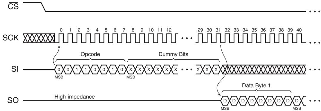
**Figure 26-7. Read Sector Protection Register Timing (Opcode 32h)**
