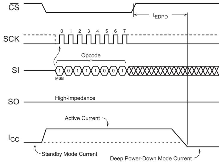
Figure 11-1. Deep Power-Down Timing
