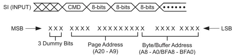
Figure 22-2. Command Sequence for Read/Write Operations for Page Size 512 bytes
