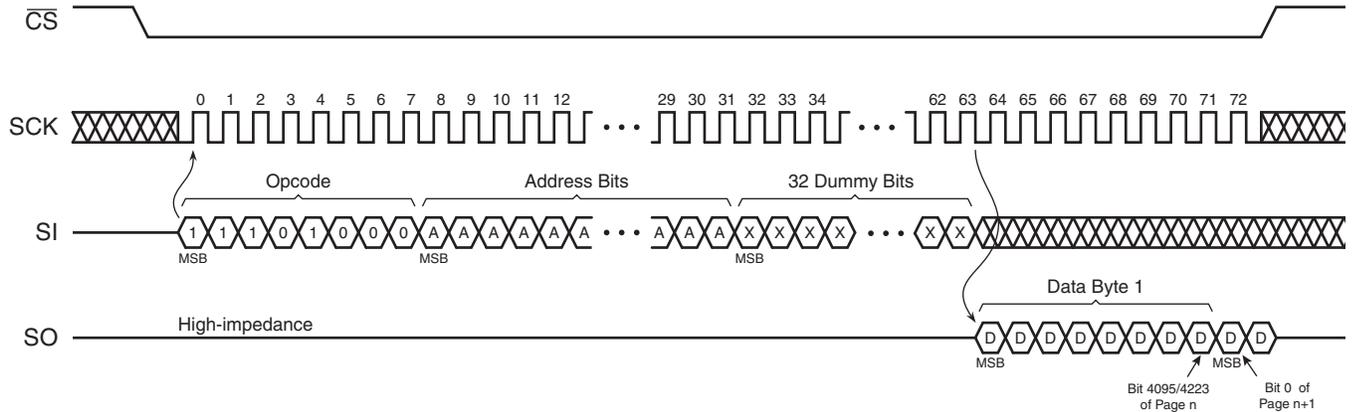
Figure 26-1. Continuous Array Read Timing (Legacy Opcode E8h)
