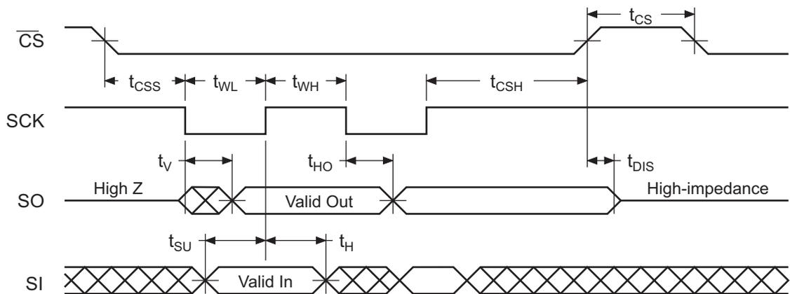
Figure 23-2. Waveform 2 = SPI Mode 3 Compatible
