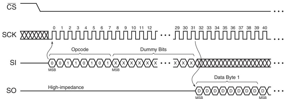
**Figure 26-8. Read Sector Lockdown Register Timing (Opcode 35h)**
