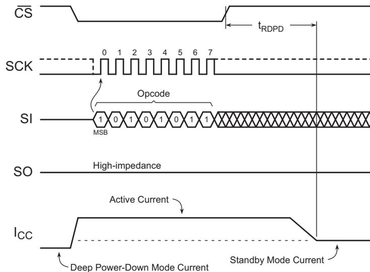
Figure 11-2. Resume from Deep Power-Down Timing
