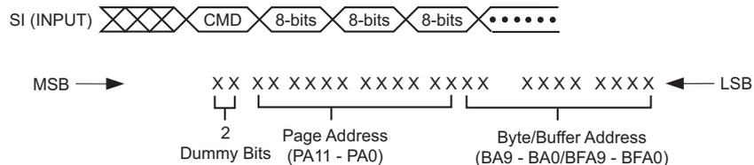
Figure 22-3. Command Sequence for Read/Write Operations for Page Size 528 bytes
