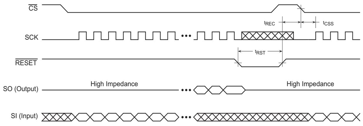
**Figure 26-12. Reset Timing**
