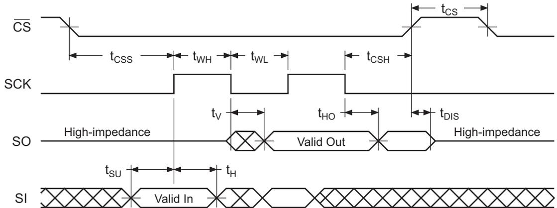
Figure 23-1. Waveform 1 = SPI Mode 0 Compatible
