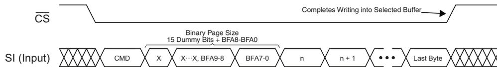
Figure 24-2. Buffer Write
